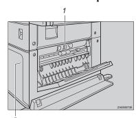
**1. Paper Feed Roller A for PS420** 2. Paper Feed Roller B,C for PS420
