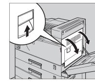
Hold the green catches of the transfer roller with both hands  $(\widehat{1})$ . Raise them to release the transfer unit (2).
