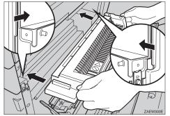
Fasten the two screws of the fusing unit.
