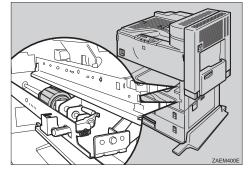
Pull the small green lever inside the printer on the lower right side.
