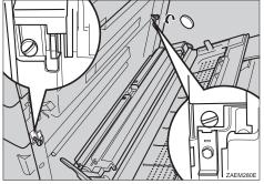
Hold the green catches with both hands and remove the fusing unit.
