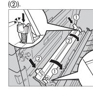
Put the transfer roller that was removed in step **3** into the plastic bag emptied in step **4**.
