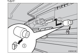
Remove the plastic bag from the new paper feed 9 rollers (B)(C) for PS420.
