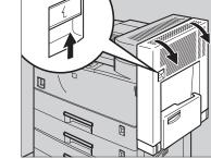
Open the right cover of the printer by lifting the catch.
