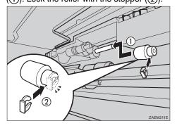
Hold the new paper feed roller (C), with its pin towards you ((1)). Insert the roller onto the front shaft until it clicks into place(2).
