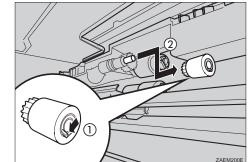
Remove the stopper from the rear paper feed roller ((1)), and remove the paper feed roller (2)
