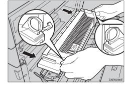
Take the new fusing unit from the box and remove the plastic bag.
