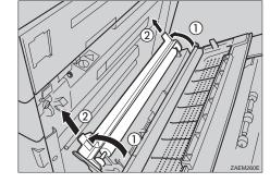
Take the new transfer roller from the box and remove the plastic bag.
