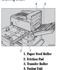
If the optional PS420 is installed, the paper feed roller for PS420 are need to be replaced.
