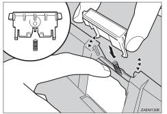
Confirm that the friction pad is properly set as shown in the illustration. If it is not properly set, reset the friction pad, following steps 10 to 12.
