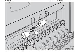
While pushing the pin of the front paper feed roller outwards ((1)), remove the paper feed roller (2).
