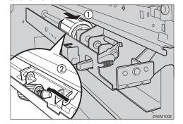
Take the new paper feed roller from the box and remove the plastic bag.
