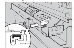
There is a paper feed roller on the lower right side inside of the printer. Push the paper feed roller (the paper feed roller of the paper tray that is second from the top) towards you (①), then pull it in a diagonally downward direction (2) and remove it.
