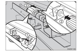
Check the motion of the paper feed roller to confirm that it is properly set.
