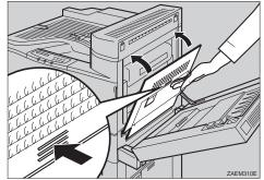
If the duplex unit is installed, close it.
